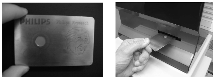
Fig. 1. Left: Card equipped with an optical PUF. Right: Reading device
