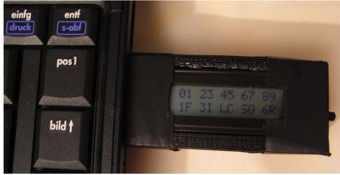
**Fig. 4.** A prototype USB token running the hPIN user authentication step.
